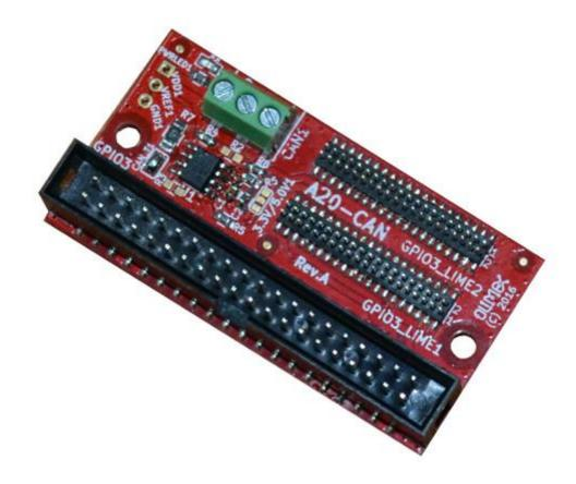
A20-CAN is CAN driver board for A20 Allwinner SOCs. A20-CAN features are:
