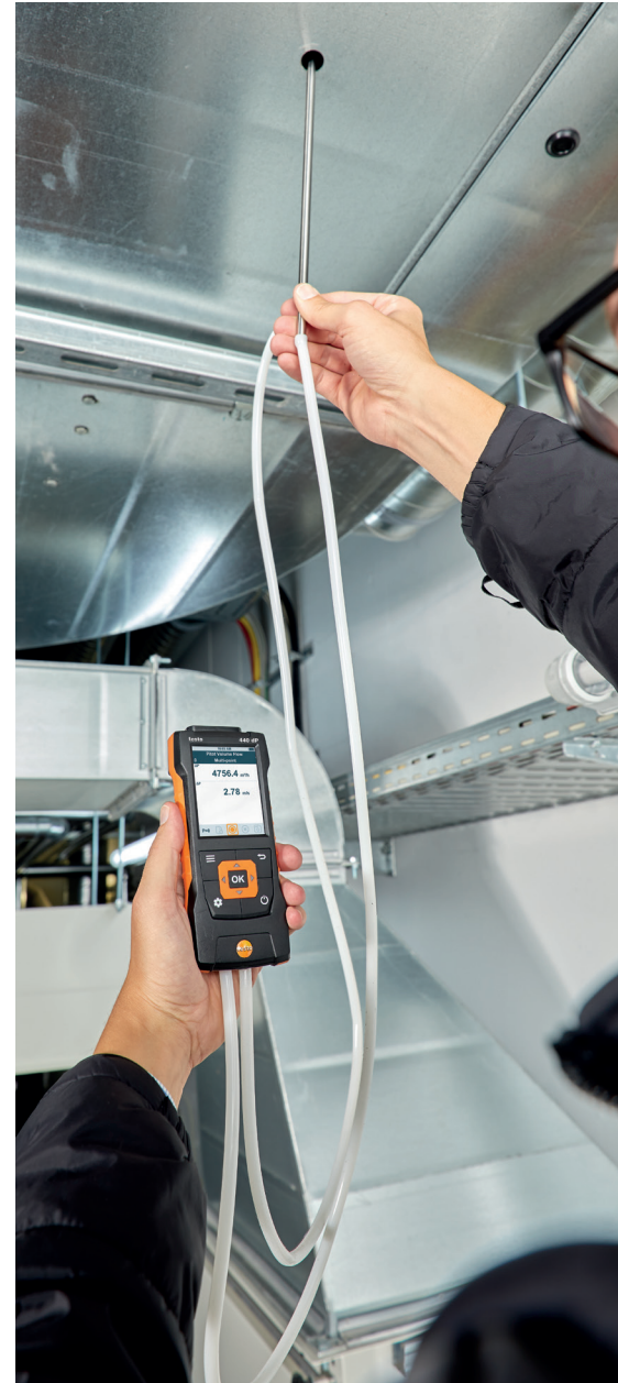
For measuring the volume flow in the case of high flow velocities or heavily contaminated flow, we recommend the testo 440 dP and a Pitot tube.
