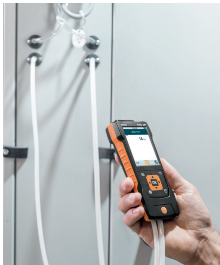
With the testo 440 dP model, incl. differential pressure sensor, you can ensure that the filters in air conditioning systems are working properly. This confirms no outdoor contamination gets indoors.
