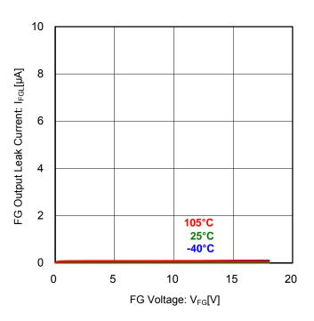
Figure 15. FG Output Leak Current vs FG Voltage
