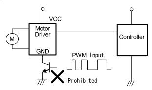
Figure 38. GND Line PWM Switching Prohibited
