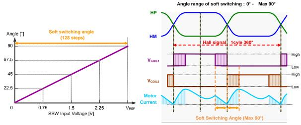
Figure 25. Relations of SSW Terminal Voltage and the Angle of Soft Switching
