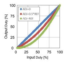
Figure 24. Input Duty vs Output Duty Characteristics
