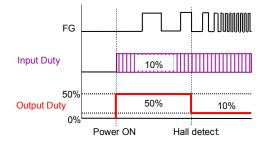
Figure 30. Start Duty Assist Operation at Input Duty 10%
