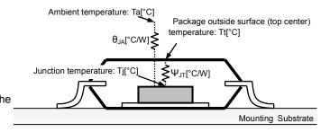
Figure 40. Thermal Resistance Model of Surface Mount
