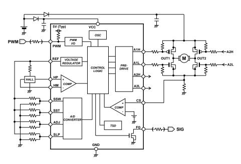
Figure 1. Application of Direct PWM Input
