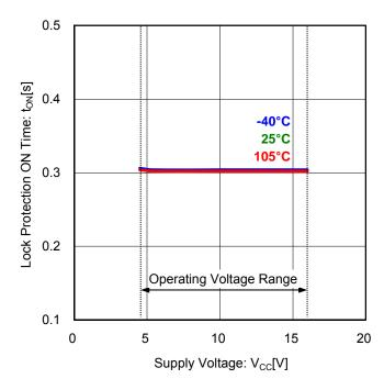
Figure 16. Lock Protection ON Time vs Supply Voltage
