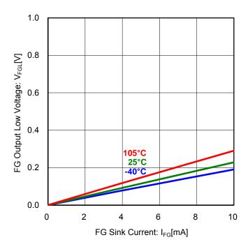
Figure 14. FG Output Low Voltage vs Sink Current
