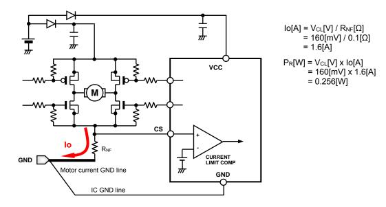
Figure 33. Current Limit Setting and GND Line
