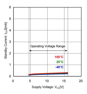
Figure 3. Standby Current vs Supply Voltage
