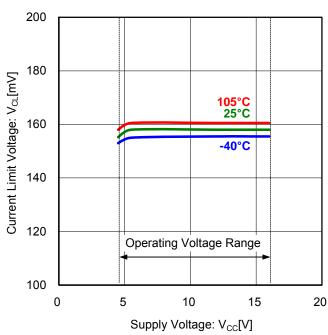
Figure 9. Current Limit Voltage vs Supply Voltage
