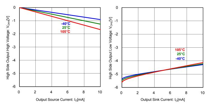
Figure 10. High Side Output High Voltage vs Source Current (V<sub>CC</sub>=12V, differential voltage to V<sub>CC</sub>)
