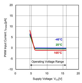
Figure 5. PWM Input Current vs Supply Voltage (V<sub>PWM</sub>=5V)
