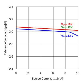
Figure 8. Reference Voltage vs Source Current (Ta=25°C)
