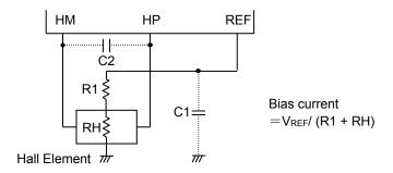
Figure 36. Application near of Hall Signal
