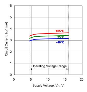
Figure 2. Circuit Current vs Supply Voltage
