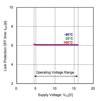
Figure 17. Lock Protection OFF Time vs Supply Voltage
