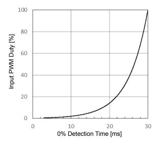
Figure 32. Input PWM Duty vs 0% Detection Time
