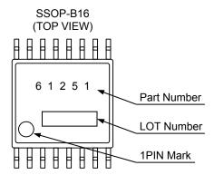
**Datasheet BD61251FV Physical Dimension Tape and Reel Information** Package Name SSOP-B16 5.  $0\pm0.2$ 16 3 2  $4\pm 0$ . 4 0  $0.15\pm0.1$  $15\pm 0$ . (UNIT:mm) PKG:SSOP-B16 0 0.65 0.  $22\pm0.1$ Drawing No. B0771 □ 0. 1 <Tape and Reel information> Tape Embossed carrier tape Quantity 2500pcs Direction The direction is the 1pin of product is at the upper left when you hold reel on the left hand and you pull out the tape on the right hand of feed
