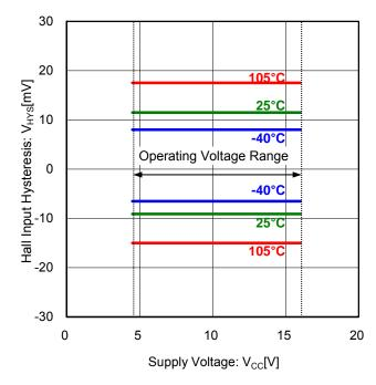
Figure 4. Hall Input Hysteresis vs Supply Voltage
