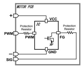
Figure 39. Protection of PWM/FG terminal
