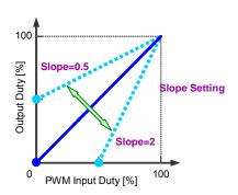
Figure 20. Properties of Input-output Duty Slope Setting
