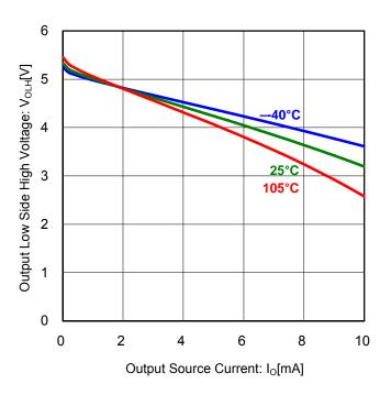
Figure 12. Low Side Output High Voltage vs Source Current (Vcc=12V)
