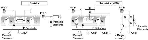
Figure 42. Example of monolithic IC structure
