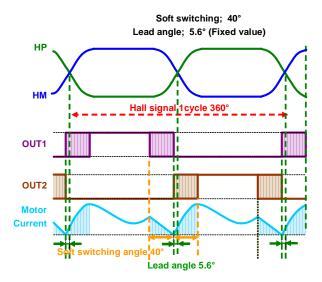
Figure 27. Lead Angle Operation
