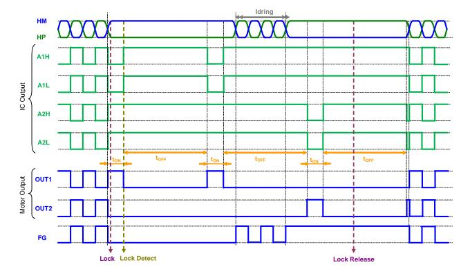
Figure 34. Lock Protection Timing Chart
