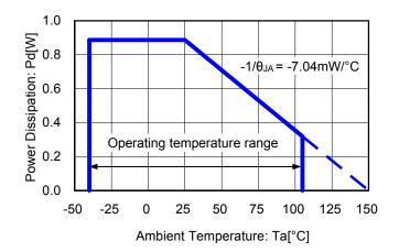
Figure 41. Power Dissipation vs Ambient Temperature
