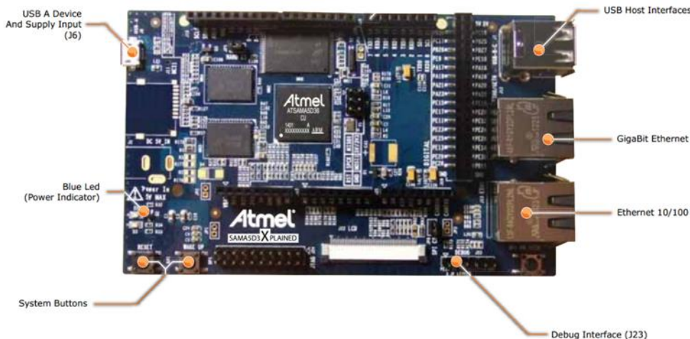
Figure 2-2. SAMA5D3 Xplained Board Overview
