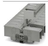
Bolt connection terminal block, Connection method: Bolt connection, Number of positions: 1, Cross section: 6 mm² - 150 mm², AWG: 10 - 300, Width: 41 mm, Color: gray, Mounting type: NS 35/7,5, NS 35/15, ct screw connection
