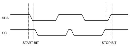
Figure 3. Start/Stop Timing
