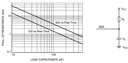
Figure 2. Pull-up Resistance vs. Load Capacitance
