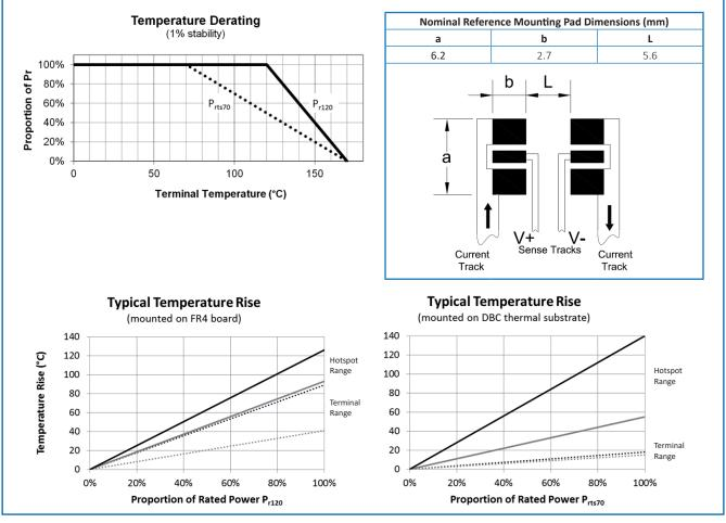
FR4 board details: 102x51mm, high T<sub>g</sub> FR4 board with 70 $\mu$ m (2 ounce) inner and outer Cu planes or similar substrate, such that terminal temperature is maintained at  $\leq$ 120°C.
