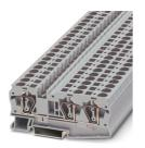
Feed-through terminal block, nom. voltage: 1000 V, nominal current: 41 A, number of connections: 3, connection method: Spring-cage connection, Rated cross section:  $6 \text{ mm}^2$ , cross section:  $0.2 \text{ mm}^2$  -  $10 \text{ mm}^2$ , mounting type: NS 35/7,5, NS 35/15, color: gray
