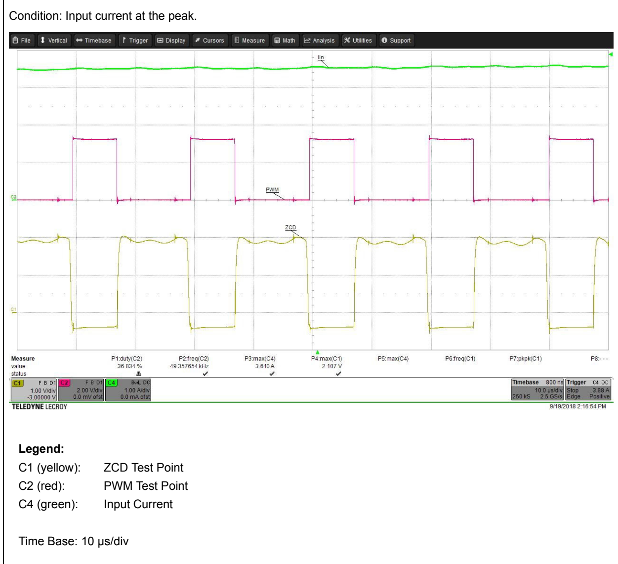
FIGURE 1-10: ZERO-CROSS DETECTION (ZCD), PWM TEST POINTS
