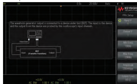
Figure 2. The FRA setup menu includes a block diagram to help you make the proper connections.
