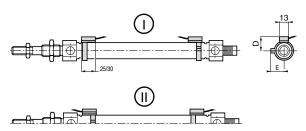
It is possible to mount magnetic detectors for intermediate position indication: mounting by collar
