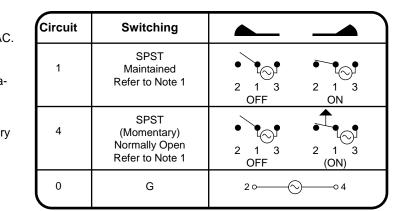
NOTE 1. Furnished with one side of the lamp internally connected and a single lamp-terminal at the back of the switch.
