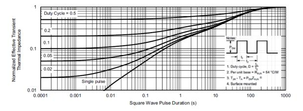
Normalized Thermal Transient Impedance, Junction-to-Ambient
