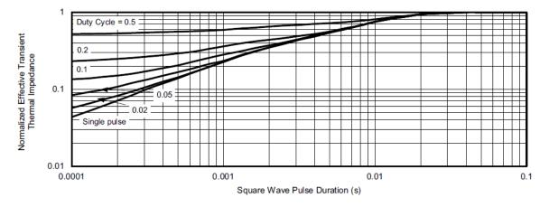
Normalized Thermal Transient Impedance, Junction-to-Case
