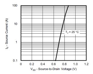
Source-Drain Diode Forward Voltage
