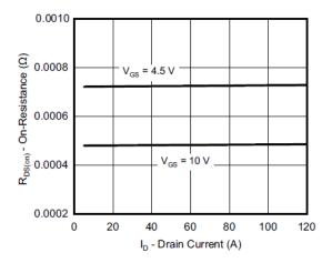
On-Resistance vs. Drain Current and Gate Voltage
