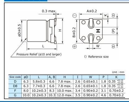
FKS-HF series (High temp. / Standard reflow)
