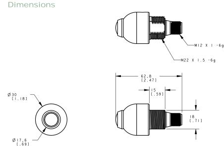
All measurements are listed in millimeters [inches], unless noted otherwise.
