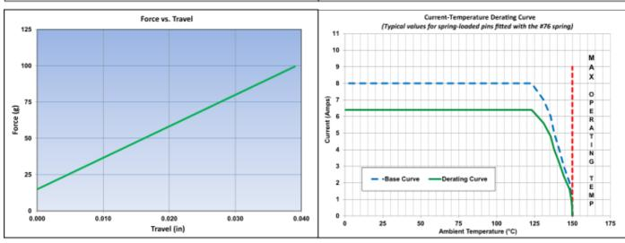
The stroke, force and current rating values are measured using spring pins with an internal construction per the design specification. Individual spring pin performance may vary from these values based on design differences.
