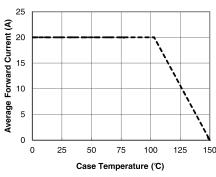
Figure 1. Forward Current Derating Curve
