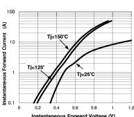
Instantaneous Forward Voltage (V) Figure 3. Typical Instantaneous Forward Characteristics Per Leg
