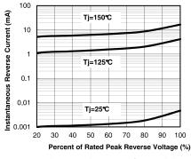
Figure 4. Typical Reverse Characteristics
