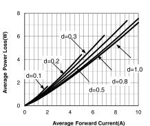
Figure 6. Forward Power Loss Characteristics
