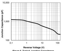
Figure 5. Typical Junction Capacitance
