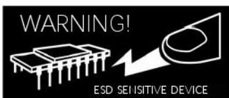
Note: This product is a static sensitive element, please pay attention to protection! ESD damage can range from subtle performance degradation to equipment failure. Precision integrated circuits may be more susceptible to damage, it can result in component parameters not meeting published specifications.
