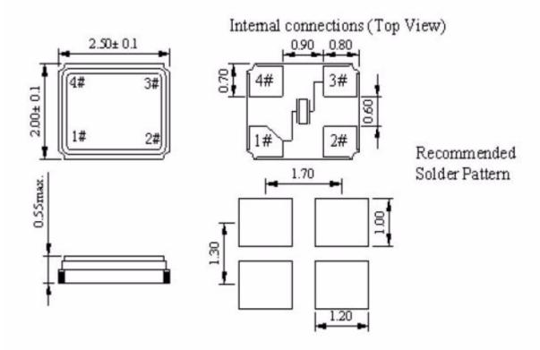
Holder Style Mode Adjustment Tolerance Temperature Stability Operating Temp. Range Load Capacitance ESR Static Capacitance (C0) Ageing Marking 25x2x05 4-pad Fundamental ± 20PPM at 25°C ± 20 PPM -30°C to +85°C 10 pF 22 Max Ohm Unspecified pF +/-2ppm/Yr Max AEL48 WW/YY
