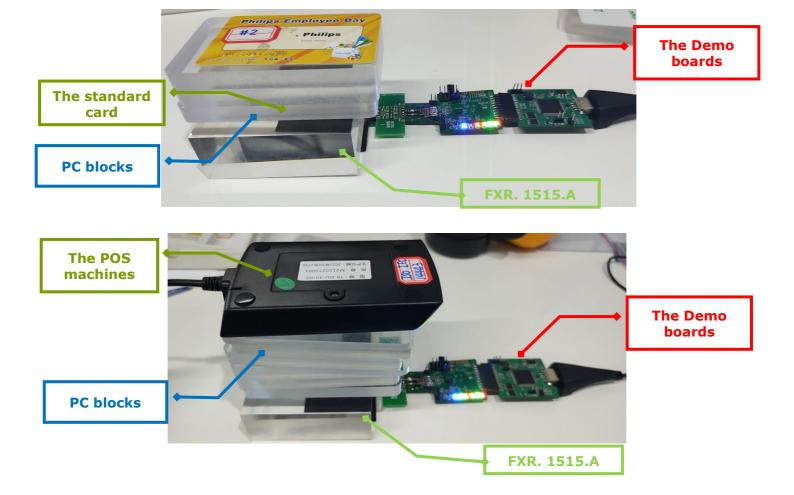
When the number of the PC material blocks are carefully adjusted until the reader can no longer read the sample, that's mean in this point the FXR.1515.A cannot establish communication with the standard card or the POS machine, the thickness of the PC material block is the maximum interrogation distance of them.
