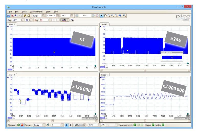
Powerful tools are included to allow you to manage and examine all of this data. As well as functions such as mask limit testing and color persistence mode, the PicoScope 6 software enables you to zoom into your waveform by several million times. The Zoom Overview window allows you to easily control the size and location of the zoom area.
