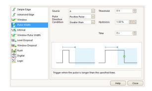
Digital triggering also reduces rearm delay and this, combined with the segmented memory, allows the triggering and capture of events that happen in rapid sequence. At the fastest timebase you can use rapid triggering to collect 10 000 waveforms in under 6 milliseconds. The mask limit testing function can then scan through these waveforms to highlight any failed waveforms for viewing in the waveform buffer.
