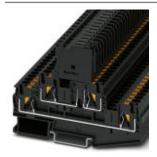
Fuse modular terminal block, Connection method: Push-in connection, Cross section: 0.2 mm²- 6 mm², AWG: 24 - 10, Nominal current: 6.3 A, Nominal voltage: 500 V, Width: 6.2 mm, Fuse type: G / 5 x 20, Fuse type: Glass / ceramics / ..., Mounting type: NS 35/7,5, NS 35/15, Color: black
