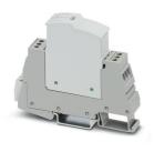
Type 3 surge protection, consisting of protective plug and base element, with integrated status indicator and remote signaling for single-phase power supply networks. Nominal voltage: 24 V AC/DC
