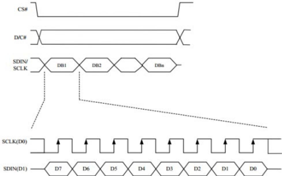
Note: Different from the traditional SPI protocol, the data line from the slave to the master is hidden since the device only has a display requirement.
