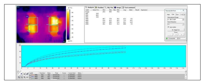
Figure 27 Peak power  $P_{out} = 225 \text{ W}$  with  $4 \Omega \text{ load } \pm 43 \text{ V}$
