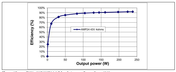
Figure 17 EVAL\_AUDAMP24 4  $\Omega$  load stereo, ±B supply = ±43 V
