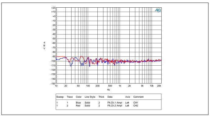
Figure 10 Noise floor 8  $\Omega$  load
