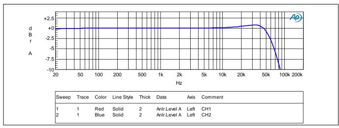
Figure 8 Frequency response 8 Ω load
