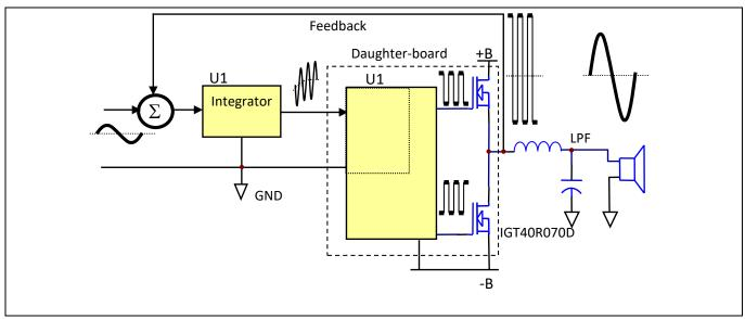
Figure 2 Simplified block diagram of class D amplifier
