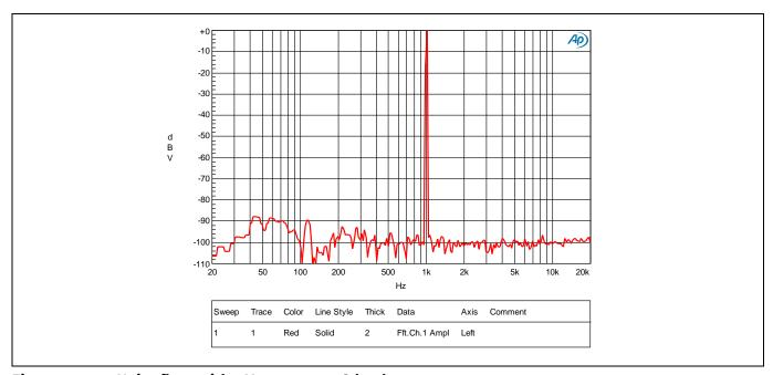
Figure 12 Noise floor with 1  $V_{RMS}$  output 8  $\Omega$  load
