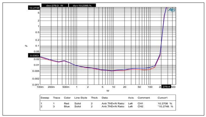
Figure 5 Power vs. THD+N 4  $\Omega$  load
