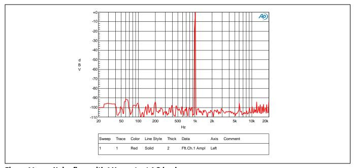
Figure 11 Noise floor with 1  $V_{RMS}$  output 4  $\Omega$  load
