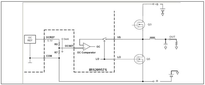
Figure 25 Simplified functional block diagram of low-side current sensing
