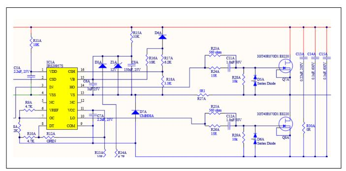
Figure 14 CoolGaN™ gate-drive interface circuit
