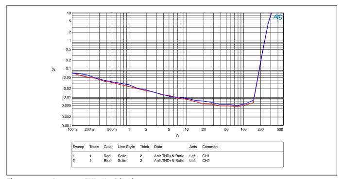
Figure 6 Power vs. THD+N 8 Ω load
