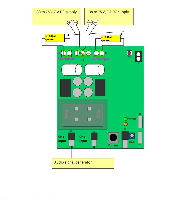
Figure 3 Typical connections
