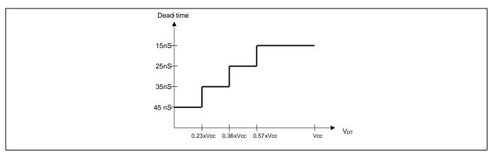
Figure 23 Dead-time setting vs. V<sub>DT</sub> voltage
