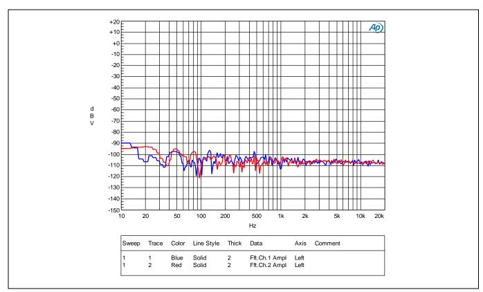
Figure 9 Noise floor  $4 \Omega$  load
