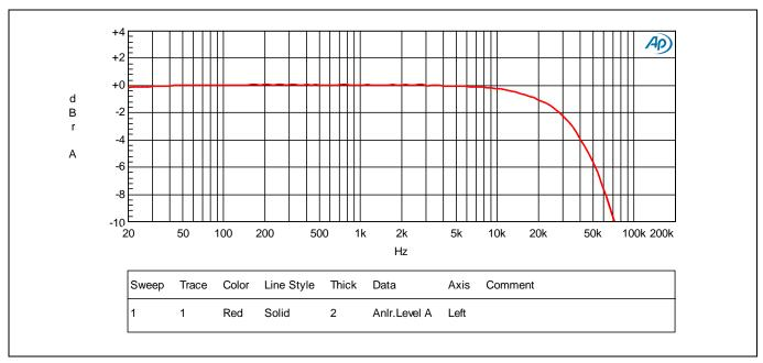
Figure 7 Frequency response 4  $\Omega$  load
