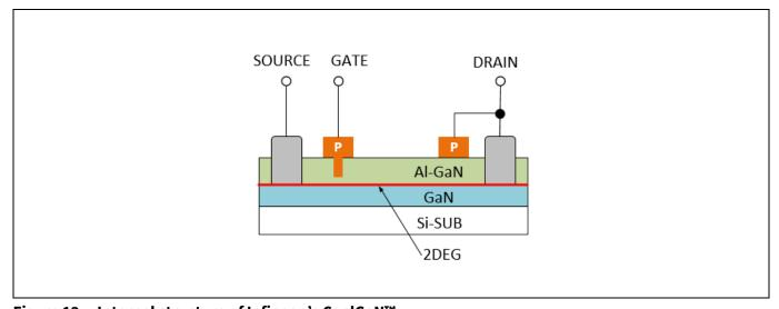
Figure 13 Internal structure of Infineon's CoolGaN™
