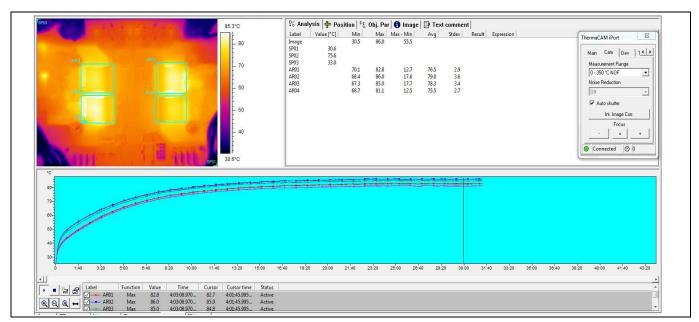
Figure 30 1/8 power = 31.25 W with 8  $\Omega$  load ±63 V
