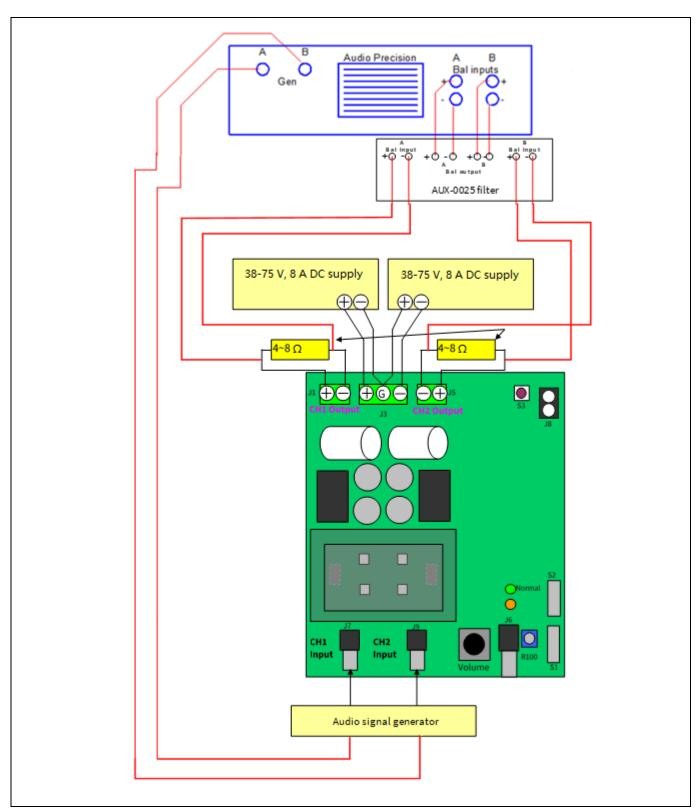
Figure 4 Audio analyzer connection
