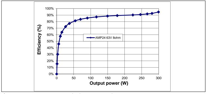
Figure 18 EVAL \_AUDAMP24 8  $\Omega$  load stereo,  $\pm$ B supply =  $\pm$ 63 V
