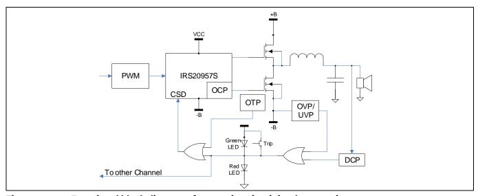
Figure 24 Functional block diagram of protection circuit implementation
