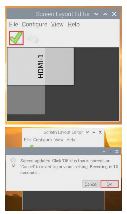
6. And then after rotating touch, the LCD can be used normally.
