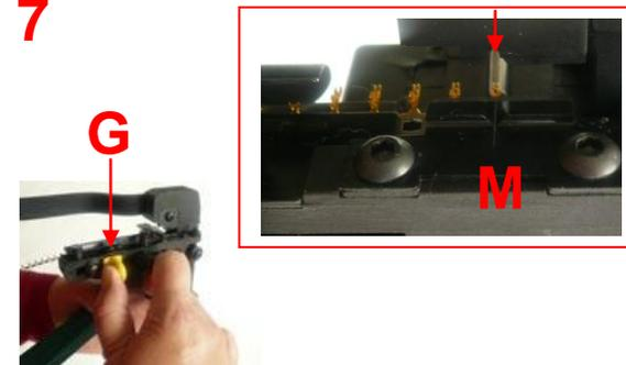
Effect the insert until contact is in the middle (M) of the crimping profile.
