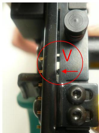
The feed pin engages with strip lock.
