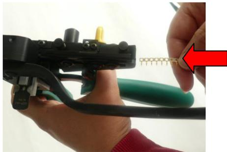
Insert the strip of contacts into the feed unit.
