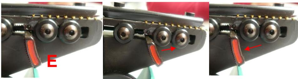
Push in until the locking lever (E) engages with the strip lock and the feed can be effected by yellow feed lever (G, see picture 7). The release lever moves automatically in direction of the arrow during the insertion of the strip of contacts.
