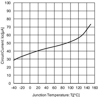
Figure 16. Circuit Current vs. Temperature
