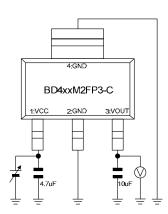
Measurement Setup for Figure 6, 8, 14, 15, Figure 24, 26, 32, 33
