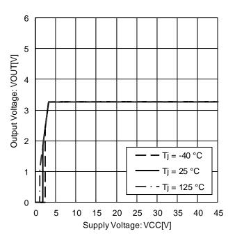
Figure 6. Output Voltage vs. Power Supply Voltage (IOUT = 0 mA)
