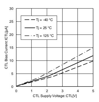
Figure 40. CTL Bias Current vs. CTL Supply Voltage
