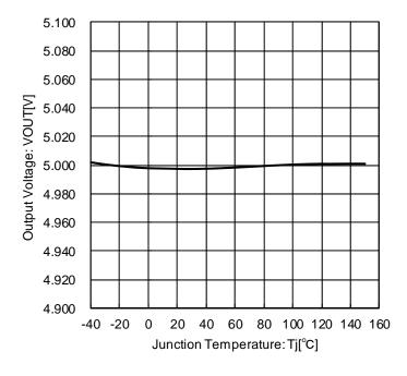
Figure 33. Output Voltage vs. Temperature
