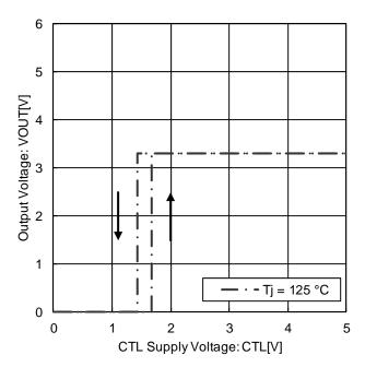
Figure 20. CTL ON / OFF Mode Voltage (Tj = 125 °C)
