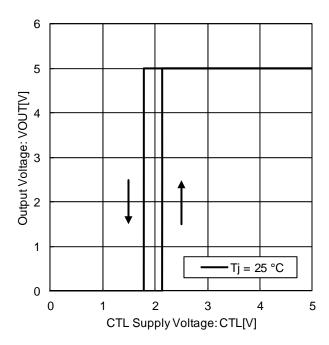
Figure 37. CTL ON / OFF Mode Voltage  $(Tj = 25 \degree C)$
