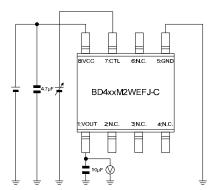
Measurement Setup for Figure 18, 19, 20, Figure 36, 37, 38
