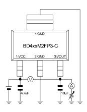
Measurement Setup for Figure 11, 29
