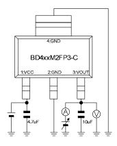
Measurement Setup for Figure 10, 28
