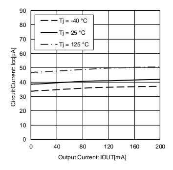
Figure 13. Circuit Current vs. Output Current
