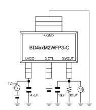
Measurement Setup for Figure 12, 30
