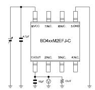
Measurement Setup for Figure 5, 7, 16, Figure 23, 25, 34
