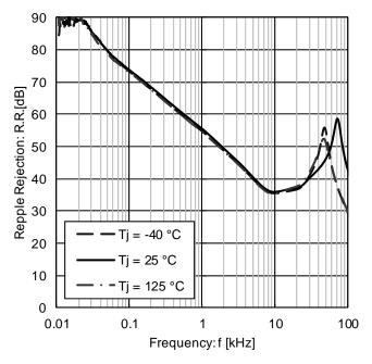
Figure 12. Ripple Rejection (ein = 1 Vrms, IOUT = 100 mA)
