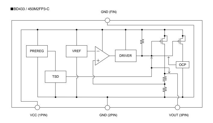
Figure 4. Block Diagrams
