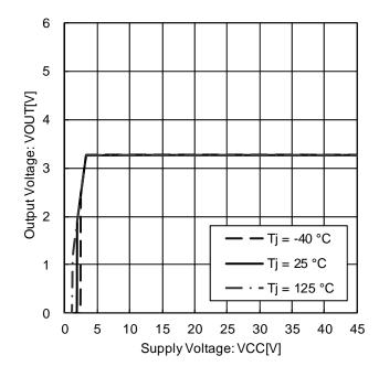
Figure 9. Output Voltage vs. Power Supply Voltage (IOUT = 10 mA)
