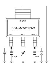
Measurement Setup for Figure 18, 19, 20, Figure 36, 37, 38
