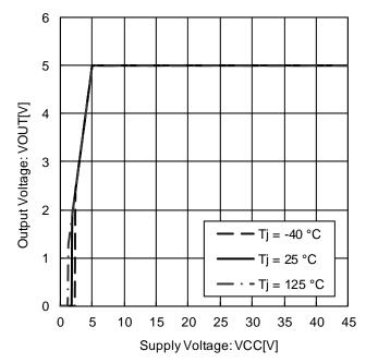
Figure 27. Output Voltage vs. Power Supply Voltage (IOUT = 10 mA)
