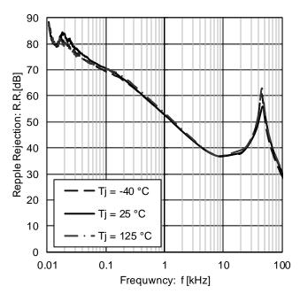
Figure 30. Ripple Rejection (ein = 1 Vrms, IOUT = 100 mA)
