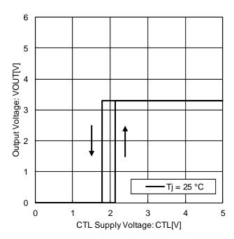
Figure 19. CTL ON / OFF Mode Voltage  $(Tj = 25 \degree C)$
