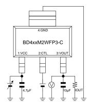
Measurement Setup for Figure 9, 27
