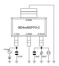
Measurement Setup for Figure 12, 30
