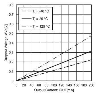
Figure 29. Dropout Voltage (VCC = 4.75 V)
