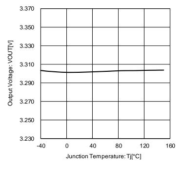
Figure 15. Output Voltage vs. Temperature
