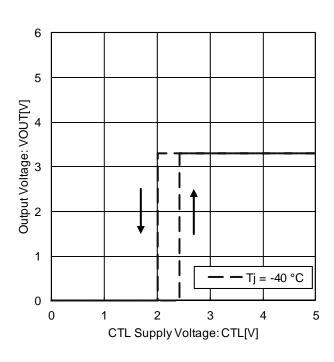
Figure 18. CTL ON / OFF Mode Voltage  $(Tj = -40 \, ^{\circ}C)$
