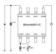
Measurement Setup for Figure 13, 31
