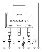
Measurement Setup for Figure 10, 28
