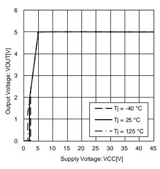
Figure 24. Output Voltage vs. Power Supply Voltage (IOUT = 0 mA)
