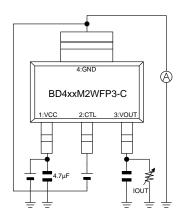
Measurement Setup for Figure 13, 31
