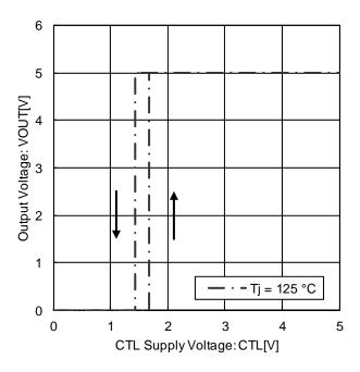
Figure 38. CTL ON / OFF Mode Voltage (Tj = 125 °C)
