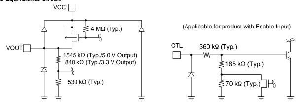
Figure 49. Input / Output Equivalence Circuit
