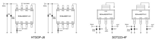
Figure 46. Sample Application Circuit 1
