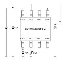
Measurement Setup for Figure 13, 31
