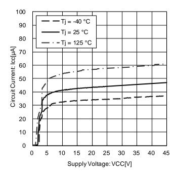
Figure 5. Circuit Current vs. Power Supply Voltage
