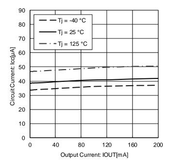
Figure 31. Circuit Current vs. Output Current
