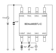
Measurement Setup for Figure 10, 28
