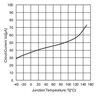
Figure 34. Circuit Current vs. Temperature
