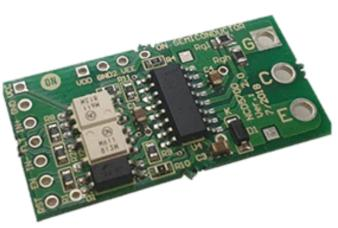
This daughter card is compatible with the SECO-GDBB-EVB gate drivers baseboard, which allows testing up to 3 half bridge daughter cards simultaneously and comparing performances.
