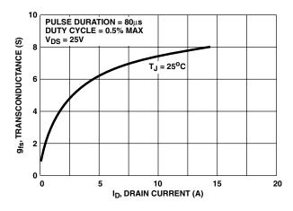
FIGURE 11. TRANSCONDUCTANCE vs DRAIN CURRENT
