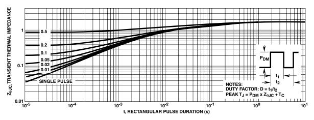
FIGURE 3. MAXIMUM TRANSIENT THERMAL IMPEDANCE
