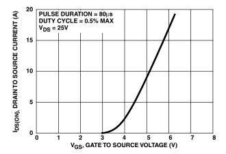
FIGURE 6. TRANSFER CHARACTERISTICS
