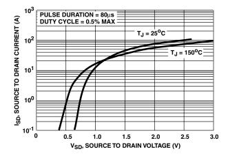
FIGURE 12. SOURCE TO DRAIN DIODE VOLTAGE
