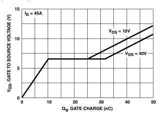
FIGURE 13. GATE TO SOURCE VOLTAGE vs GATE CHARGE
