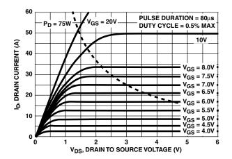
FIGURE 5. OUTPUT CHARACTERISTICS
