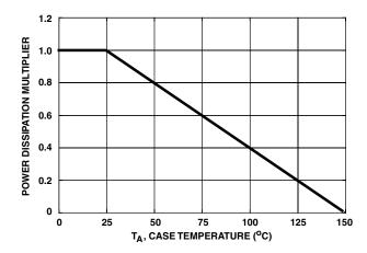
FIGURE 1. NORMALIZED POWER DISSIPATION vs CASE TEMPERATURE
