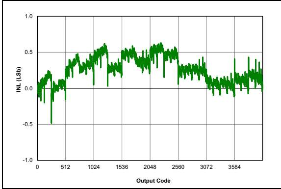
FIGURE 45-97: ADC 12-bit Mode, Single-Ended INL, V_{DD} = 2.3V , V_{REF} = 2.3V , T_{AD} = 1 \mu S , CP ON, 25°C.
