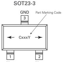
Part Marking Code: Cxxxy: C = LF22214TMR; xxx = Julian manufactured date; y = manufactured year Moisture Sensitivity Level: Rating is 3
