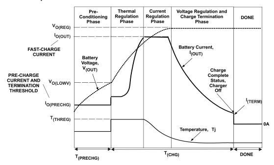
Figure 5. Charging Profile With Thermal Regulation
