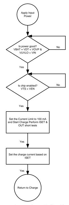
Figure 7. bq21040 Power-Up Flow Diagram
