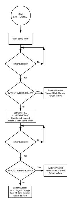
Figure 9. Battery Detect Routine (bq21040)
