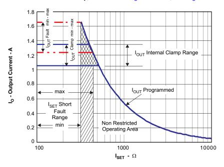
Figure 8. Programmed/Clamped Out Current
