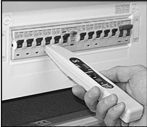
Figure 4. Correct The receiver must be held in this orientation in relation to the breaker to find the correct fuse/circuit breaker. If the individual breakers were horizontal, the receiver would have to be rotated through 90° (in either direction).
