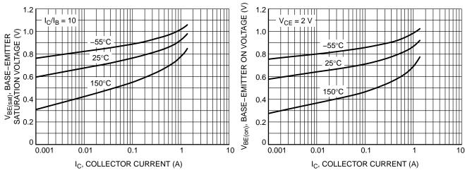
Figure 3. Base-Emitter Saturation Voltage
