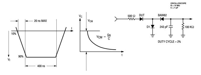
Figure 2. Stored Charge Equivalent Test Circuit
