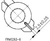
Hole arrangement View in mounting direction
