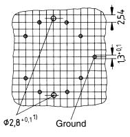
Hole arrangement View in mounting direction
