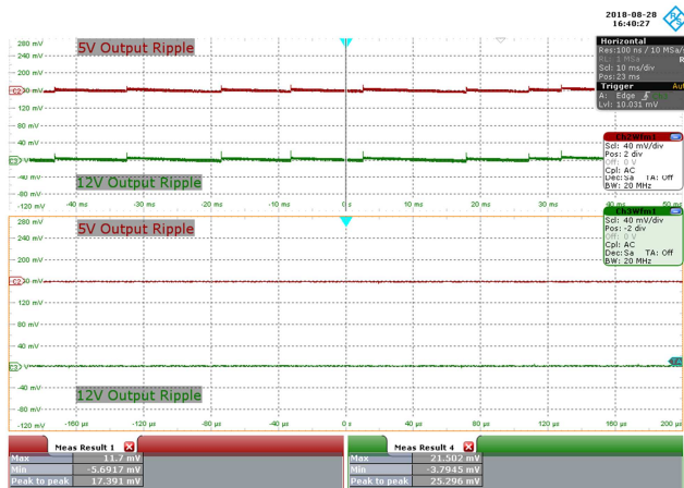
Figure 126 – 85 VAC 60 Hz, 0% Load. CH2: 5 V OUT , 40 mV / div., 10 ms / div. CH3: 12 V OUT , 40 mV / div., 10 ms / div. Zoom: 40 µs / div. 5 V Output Ripple = 17.391 mV. 12 V Output Ripple = 25.296 mV.
