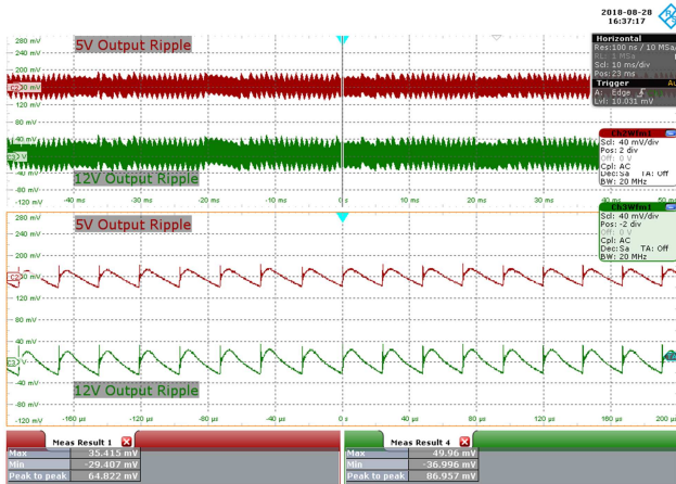
Figure 118 – 85 VAC 60 Hz, 50% Load. CH2: 5 V OUT , 40 mV / div., 10 ms / div. CH3: 12 V OUT , 40 mV / div., 10 ms / div. Zoom: 40 μs / div. 5 V Output Ripple = 64.822 mV. 12 V Output Ripple = 86.957 mV.
