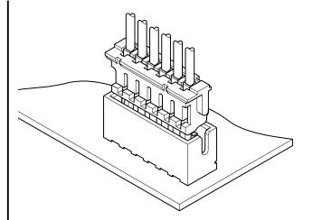
The ZH connector is very small with a mounting height of 5.6 mm and a thickness of only 3.5 mm. Contact retention lances on the housing make insertion easier, while the dimple at the center of the contact ensures reliable contact with the post.
