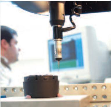
Checking the injection moulded parts with the assistance of a 3D coordinate measuring machine.
