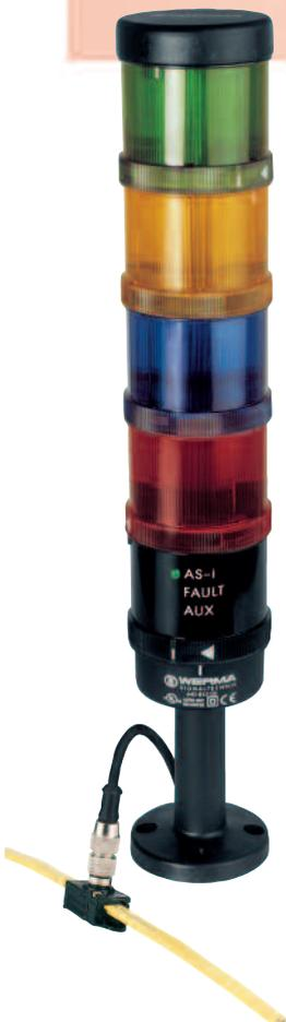
The new AS Interface Element is available with either Standard Slave or the new A/B technology. The Standard Slave models are, as specified by AS Interface specification 2.11, able to address up to 31 modules and trigger four tiers. The new A/B technology makes it possible to address up to 62 modules and trigger three tiers.
