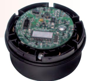
Many applications require the signalisation of the current operating status even when a PLC or control system is not available. The new terminal element with USB interface is easy to activate as it is triggered directly via a PC.
