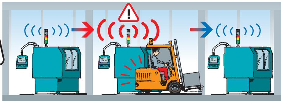
The siren element adjusts its sound output through continual measurement of the ambient noise level. The emitted tone is c. 5 dB louder than the background sound level. The warning signal can always be heard without being irritatingly loud for people in the sounder's vicinity.
