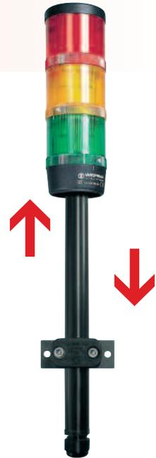
The tube with clamp, for example, offers the possibility of varying the height of the mounted KombiSIGN signal tower. In addition, it allows the signal tower to be removed whilst remaining connected. This feature is particularly beneficial when the machinery including the signal tower has to be transported.
