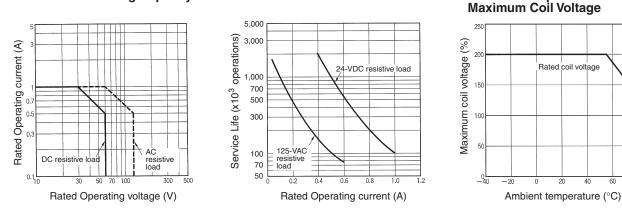
**Note:** The maximum coil voltage refers to the maximum value in a varying range of operating power voltage, not a continuous voltage.
