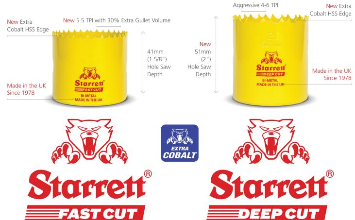
The new Fast Cut Bi-Metal Hole Saws contain an extra cobalt HSS tooth material for enhanced heat and wear resistance, along with a new 5.5 TPI positive rake tooth design, to ensure a smoother and faster cut when compared against our previous Constant Pitch Hole Saw. Specifically designed to cut stainless steel, metals and mild steel sheet, the Fast Cut Saws will also cut through wood, plastic, plaster and other materials.
