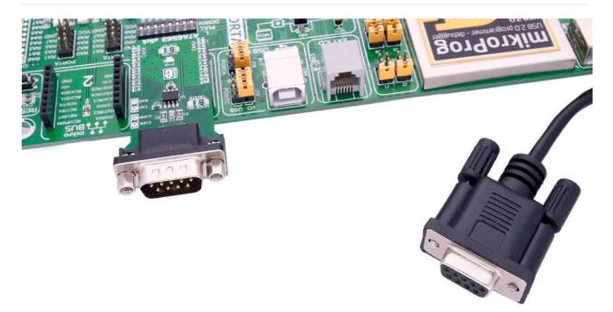
ATA6563 click is connected to a CAN bus via the DB9 cable, which then communicates with the network.
