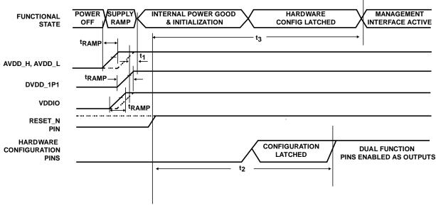
Figure 2. Power-Up Timing
