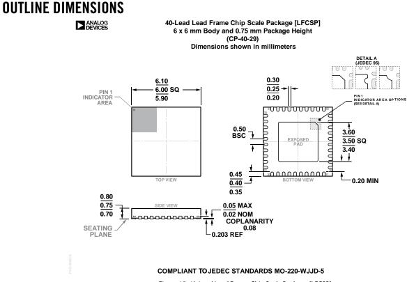
Figure 15. 40-Lead Lead Frame Chip Scale Package [LFCSP] 6 mm x 6 mm Body and 0.75 mm Package Height (CP-40-29). Dimensions shown in millimeters
