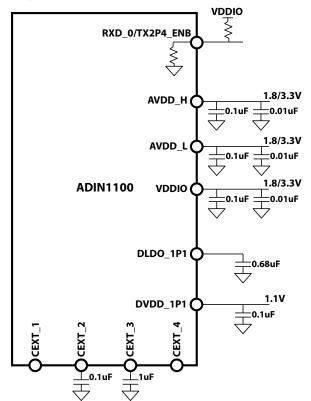
Figure 10. Supplies and capacitors for forced 1V pk-pk transmit mode
