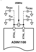
Figure 13. Crystal Oscillator Connection
