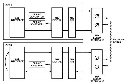
Figure 9. Remote Loopback used across Two PHYs for Self Check Purposes
