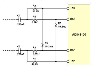
Figure 7. Recommended hybrid for the ADIN1100.
