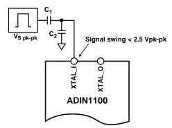
Figure 14. External Clock Connection
