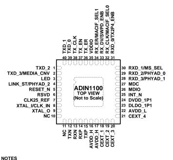
1. EXPOSED PAD. THE LFCSP HAS AN EXPOSED PAD THAT MUST BE SOLDERED TO A METAL PLATE ON THE PCB FOR MECHANICAL REASONS AND TO GND.
