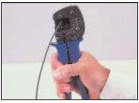
With the terminal and wire set in the proper position, (see above) hold the wire stationary and squeeze the tool together. Complete the crimp by squeezing the tool until the ratchet releases. Remove the terminated wire from the tool.
