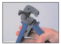
With hand tool in ready position, (open handle) open the terminal receptacle.
