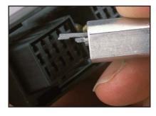
Hold connector with cavity letter and number identification in the upright position. Terminal removal tool is to be inserted in the front of the cavity, opposite to the wires.
