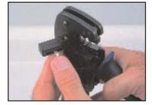
Insert an individual terminal into the proper window as directed by wire gauge indicators on the tool.
