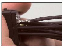
Remove the tool from the connector. Pull the wire out.
