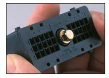
Secure the insulator in place by holding it in one hand. Make sure that Cavity Identification letters are in the upright position. (Shown below).
