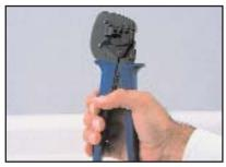
Grip the hand crimp tool securely and squeeze, ratcheting the mechanism until it bottoms out. Then allow it to open completely.
