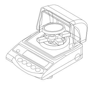
Screw the bracket on tightly according to the drawing and subsequently attach the weighing plate.
