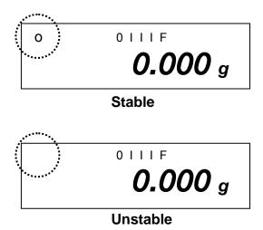
The balance is in a stable condition if the [o] stability indication appears on the display. The [o] indication disappears if the condition is unstable.
