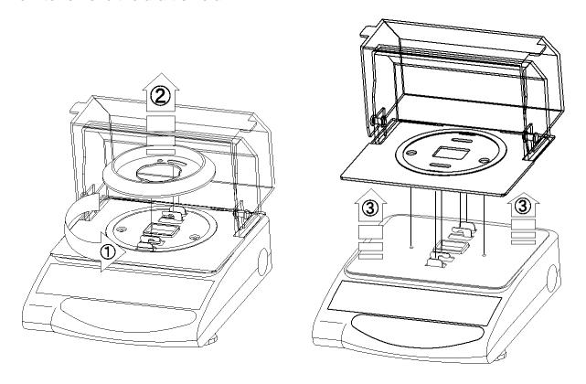
Release both retaining hooks on the lower housing section and carefully remove the lower housing section to the rear (please observe the upper housing section guides on the back of the balance).
