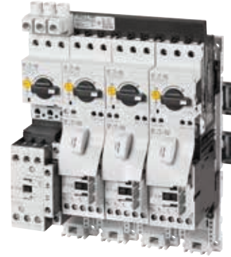
Photo 5: Examples of UL 508 Type F Combination Starters, which consist of UL 508 manual self-protected Type E Combination controllers combined with standard magnetic contactors.
