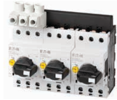
Photo 4: A PKZM0 motor protective starter grouping is linked on its supply side via a 3 phase bus connector bus. The motor protectors are fed using a common incoming terminal block BK25...-E, which features larger, distribution size electrical clearances to fulfill the requirements of a "Type E construction":
