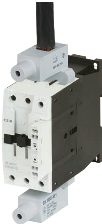
Photo 9: The paralleling bridge allows the AC-1 "General Purpose" 3 phase current rating of the contactor to be increased by a factor 2.5 times its value. This accessory is especially useful when switching single phase resistive loads (such as heaters). It permits the use of smaller, and more economical, contactors to handle the load.
