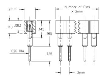
Description: Interconnect Socket 2mm Grid; Straight Socket Single Row Through Hole Accepts .015-.025" Leads Plating Code: 43 Shell Plating: 200 μ" Tin (matte finish) over 100 μ" Nickel Inner Contact Plating: 30 μ" Gold over 50 μ" Nickel
