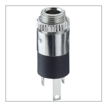
Jack chassis socket acc. to JIS C 6560 JC35J3A, 3.5 mm, 3 poles/stereo, with solder eyes, for printed circuit boards, for back side mounting
